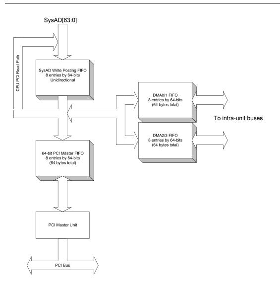
If the GT-96100A is configured to have two 32-bit PCI interfaces, then each master interface includes its own FIFO of eight entries, each 64-bits wide, see Figure 26. During writes to the PCI interface, the target PCI unit receives write data from the CPU interface or the DMA unit. When the PCI bus is granted, the PCI master's FIFO delivers the write data to the target on the PCI bus.
