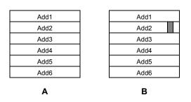
In case A where Add1-6 has the same Hash function, and thus start with the same tblEntry, the CPU allocates them in the table by increasing tblEntry by one entry each time. Add1 is the first address to be written into the table and Add6 is the last.
