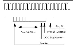
At the end of a frame there are 1-2 stop bits before the transmitter can start to transmit the next frame. If there is nothing to transmit, a continuous '1' is transmitted. This indicates that the line is idle.
