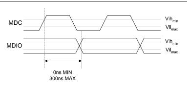
Figure 51: MDIO Setup and Hold Time
