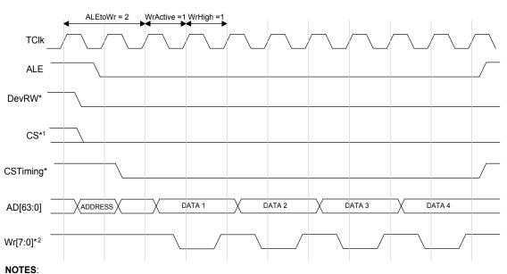
Figure 21: Waveform Showing Device Write Parameters
