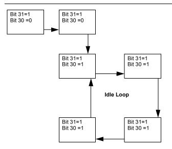
Figure 56: Using Auto Mode to Create Idle Loop
