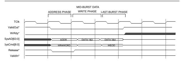
Figure 9: CPU Four Word Burst Write
