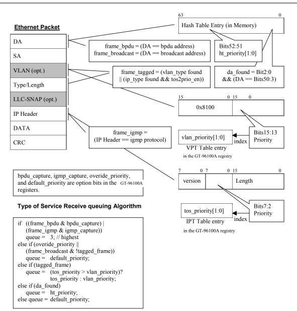
Figure 43: Type of Service Queueing Algorithm
