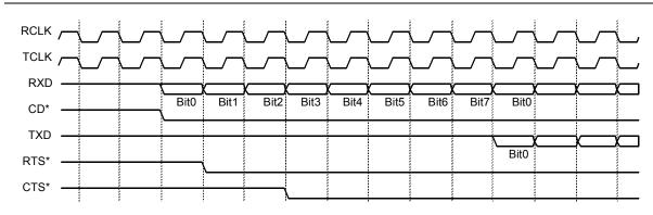
Figure 104:Transmit Synchronize to Receive (TSYN=1 in MMCRLx), External Sync (RSYL=0 in MMCRHx), CD\* and CTS\* Pulse Mode (CTSM=1 and CDM=1 in MMCRLx), Synchronous CTS\* (CTSS=1 in MMCRLx) Waveform
