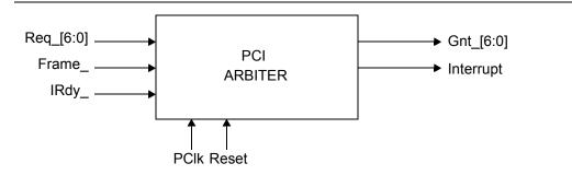
Figure 33: PCI Arbiter's Interface Diagram
