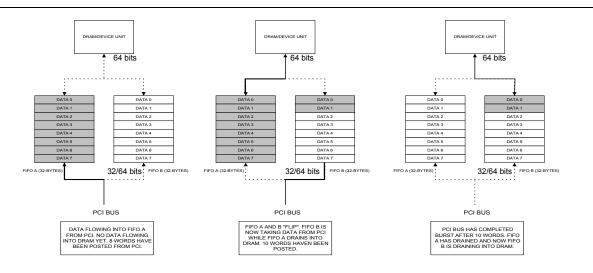
Figure 28: PCI Target Interface FIFOs Operational Example
