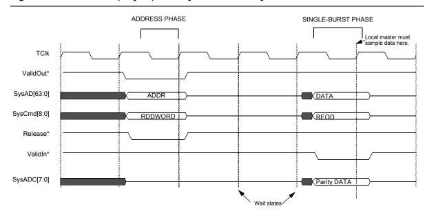
Figure 7: Double Word (8 bytes) Read by CPU With Parity Check Bits
