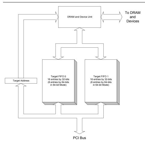
Figure 27: PCI Target Interface "Ping-Pong" FIFOs
