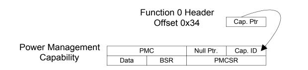
The GT-96100A supports Power Management through reset configuration pins SDQM[1:0], each pin per each PCI interface.
